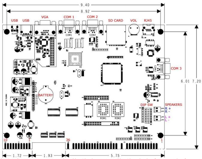
Caution: there are components on the solder side; do not press solder side on hard surface or metal surface; elevate the board about ½ inch from surface.
