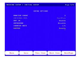
When using hopper function, must set "enable" for hopper
